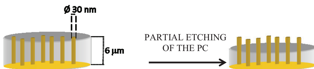
Figure 1.9. Schematic drawing of the effect of the etching on the NEE structure.
