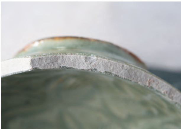
Fig. 12. Yaozhou greenware fragment showing a white layer of anorthite crystals at the body-glaze interface, Northern Song (960–1127) or Jin dynasty (1115–1234), Yaozhou Kiln Museum. Photo by the author.
