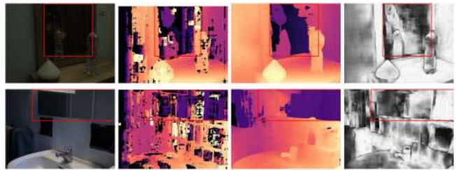
Fig. 12. Qualitative examples on the Booster [110] dataset. From left to right: RGB image, disparity map computed using the SGM algorithm, refined disparity map using our refinement method, and finally, the aleatoric confidence estimated by our network.
