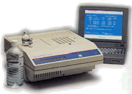
Figure 3.8 (a) Instrument utilized for Microtox ® test; (b) Vibrio fischeri .
