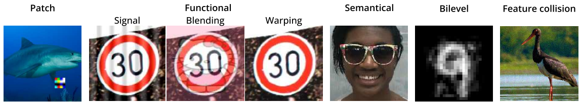
Fig. 3.2: Visual examples of data perturbation noise. The first four figures show some examples of patch, functional, and semantical triggers. For functional triggers we consider signal [15], blending [50], and warping [205] transformations. The remaining two depict poisoning samples crafted with a bilevel attack with visible noise, and a clean-label feature collision attack with imperceptible noise.
