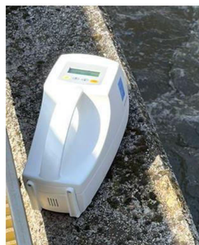
Portable pump for gelatine filters at wastewater aeration tank Sartorius MD8 AirPort
