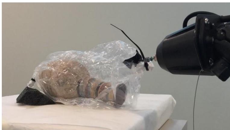
Figure 1. In museum SIFT measurement of the headspace of an amphora inside the nalophan bag (credit ME Torino).
