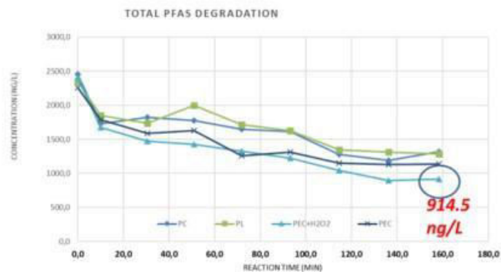
Fig.1 – Degradation of L-PFOS in real contaminated groundwater by UV-based processes.
