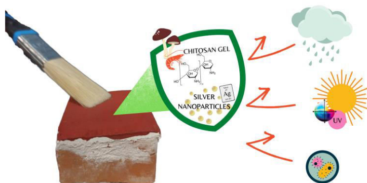
Green coating for protection of roman frescoes exposed outdoor
