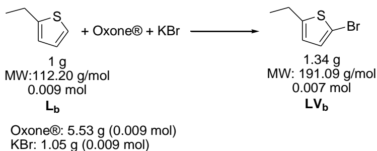
Scheme 3.9.15. Bromination of L b by using KBr/Oxone®
