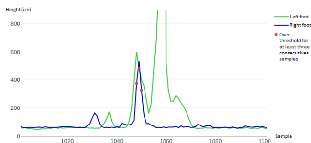
Figure 13. A zoom-in of the third (rightmost) double Lutz of the series of three in Figure 12. After the flying phase, marked by the three red dots and regularly detected as a valid jump, the left foot went parallel to the ground, hence the high green peak reaching the hard limit of the laser sensor, whereas the right foot (blue line) remained on the ground. This scenario corresponded to the exit phase of the element and was not detected as a jump.
