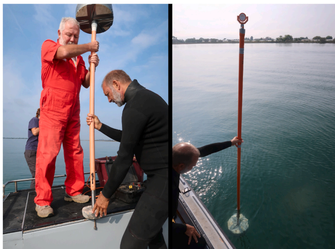
Fig. 5. The long pole with the prism employed for the topographic survey.
