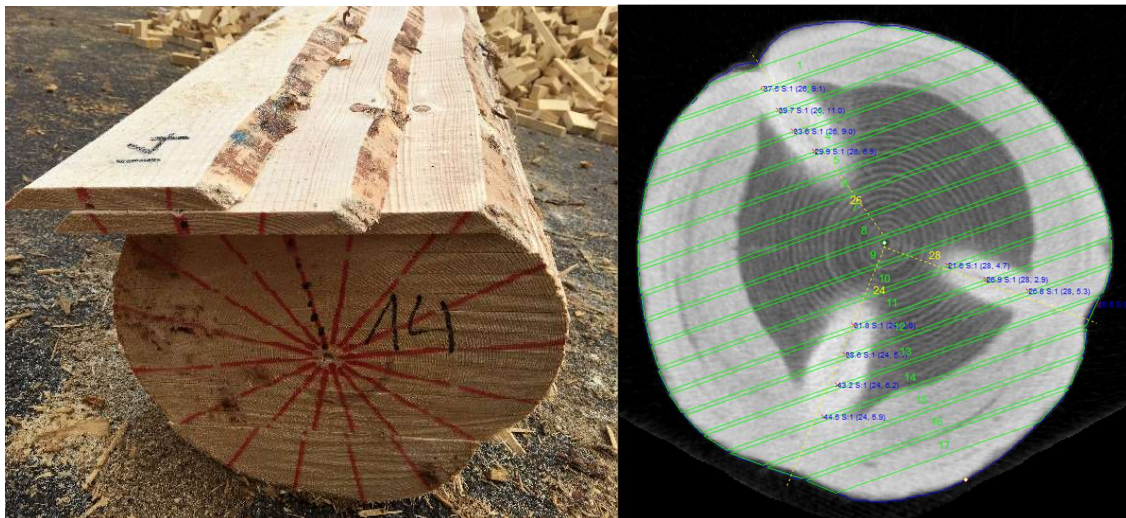
Figure 5 — An example of reference taken on a log that is CT-scanned and then sawn in boards (left), the manual measurements superimposed on the CT image (right).
