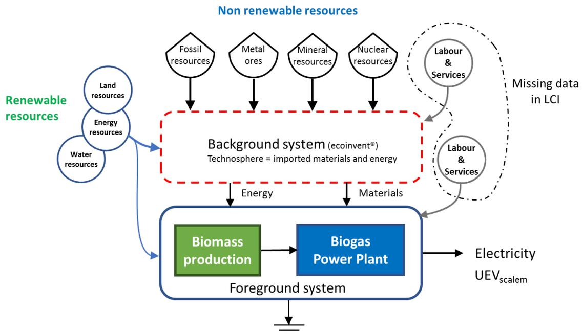
Figure 4. Graphical representation of SCALEM® energy evaluation.
