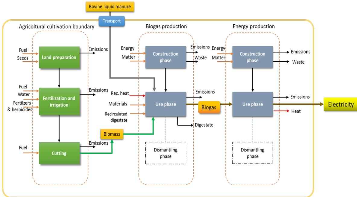
Figure 3. Life cycle flowchart for the biogas power plant.
