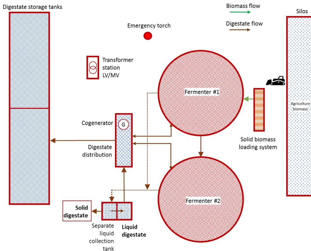
**Figure 1.** Schematic description of the biogas power plant analyzed with biomass and digestate flows.
