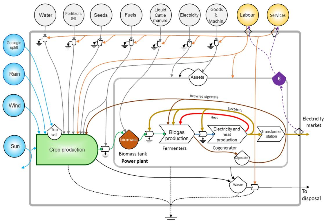
**Figure 2.** Energy system diagram of the biogas power plant, including the biomass cultivation.
