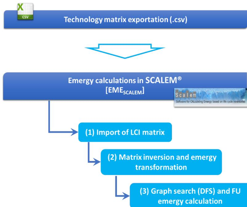
**Figure 5.** Schematic procedure of calculation made by the software SCALEM®.
