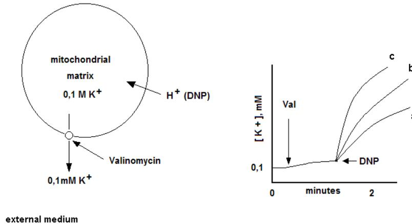
**Figure 6:** Mechanism of DNP toxicity. In non respiring mitochondria the rate of  $K^+$  efflux (in the presence of valinomycin) is proportional to DNP concentration. A similar response is obtained with the  $(\text{alkyl})_3\text{Sn}$ - compounds, thus demonstrating that they are protonophores. In a,  $[\text{DNP}] = 10 \mu\text{M}$ , in b,  $[\text{DNP}] = 20 \mu\text{M}$ , in c,  $[\text{DNP}] = 30 \mu\text{M}$ .
