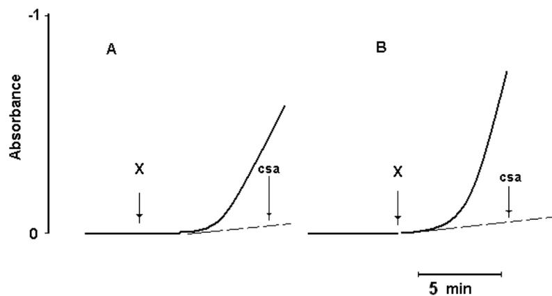
**Figure 7:** Spectrophotometrical measurement of mitochondrial swelling. The mitochondrial swelling is monitorable as absorbance decrease at 540 nm. The phenomenon is time-delayed and depends on the inducer concentration. The figure shows a typical experiment with two concentrations of the same inducer (X):  $[\text{X}]_B > [\text{X}]_A$  are used. In the case of  $(\text{alkyl})_3\text{Sn}$ - compounds, the response is cyclosporine-sensitive (csa) (dotted line).
