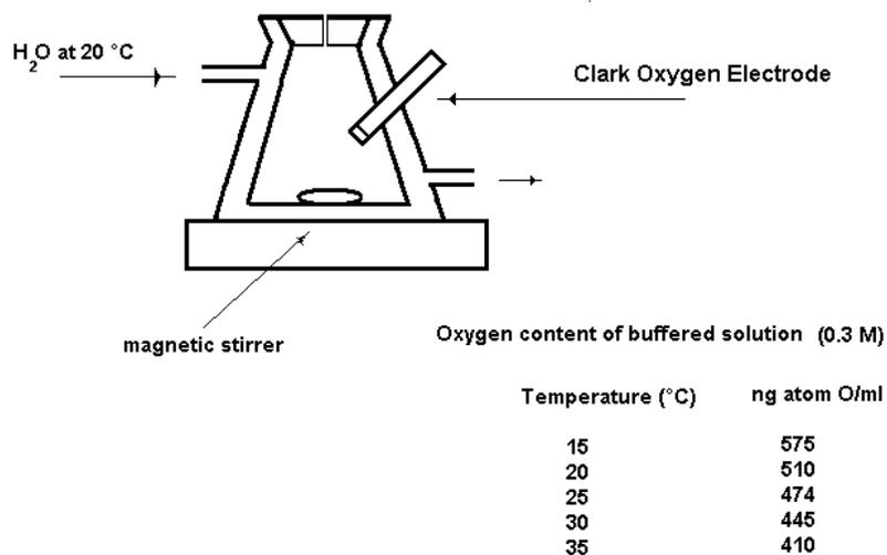
Figure 1: The rate of oxygen consumption in mitochondria can be followed by means of a selective oxygen electrode (Clark electrode).
