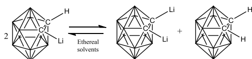
Scheme 1. The equilibrium between the species involved in the reaction of 1,2-C 2 B 10 H 12 with nBuLi.
