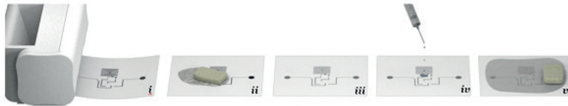
Fig.1 Step-By-Step production of stretchable circuits over the tattoo or transfer paper. Laser Printing(i), followed by coating with Ag based epoxy, and Eutectic alloy of Gallium and Indium
