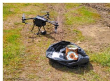
Fig. 1 Field tests: "M6" near radiation source detecting gamma radiation
