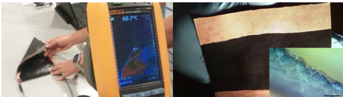
Fig.1 Left image: Flexible heating device with homogeneous temperature distribution based on an electrically con-
