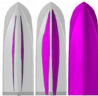
Fig.1 Optimized infusion strategy: resin front advance.
