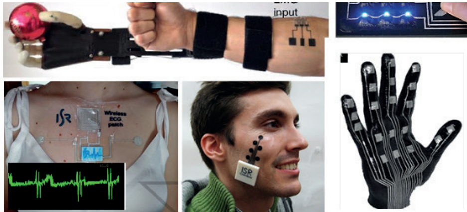
Fig.2 Applications of the electronic tattoo in EMG/ECG monitoring, and novel forms of Human Machine Interfaces
