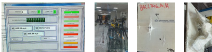
Fig.3 Ballistic test: a) Measurement Software, b) Front View, and c) and d) Back view.
