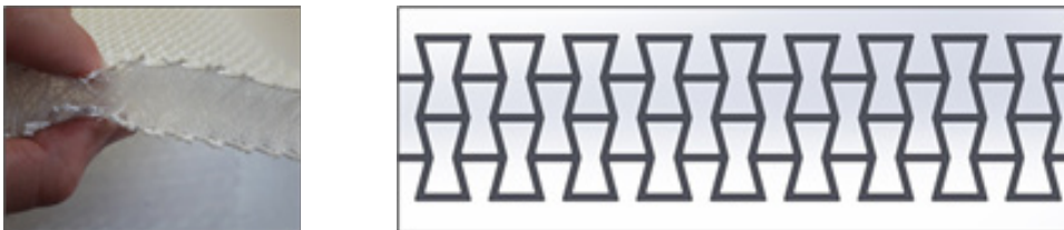
Fig.2 Example of a 3D fabric (left) and scheme of the auxetic structure used in the project (right).
