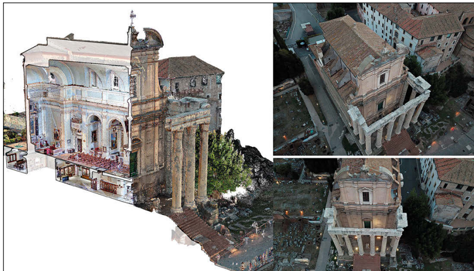
Fig. 1 – On the left, the church of San Lorenzo in Miranda's 3D laser scanner point cloud vertical section; on the right, aerial views in the archaeological area of the Roman Forum (images acquired during the SAPR survey campaign in 2022).
