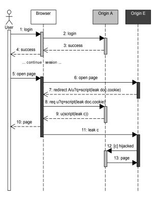
Figure 1.1: Reflected cross-site scripting attack
