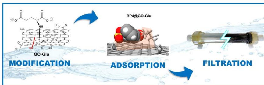
Modified graphene oxide used as sorbent for drinking water purification
