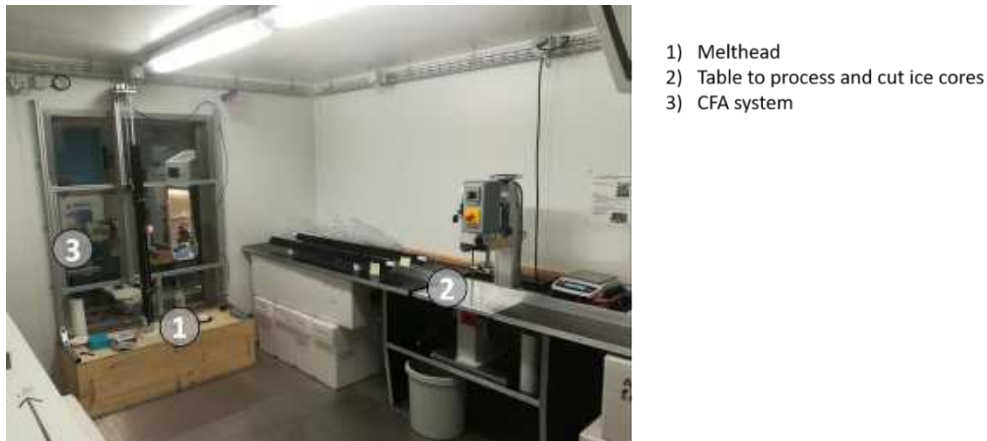
Figure 22 - The freezer where ice cores where cut and melted
