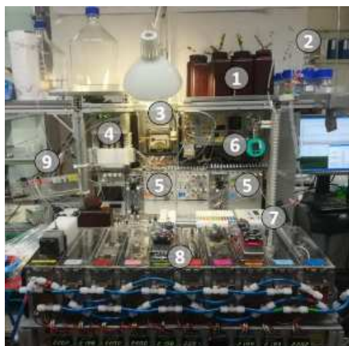
Figure 21 - The Bern CFA system: real view
