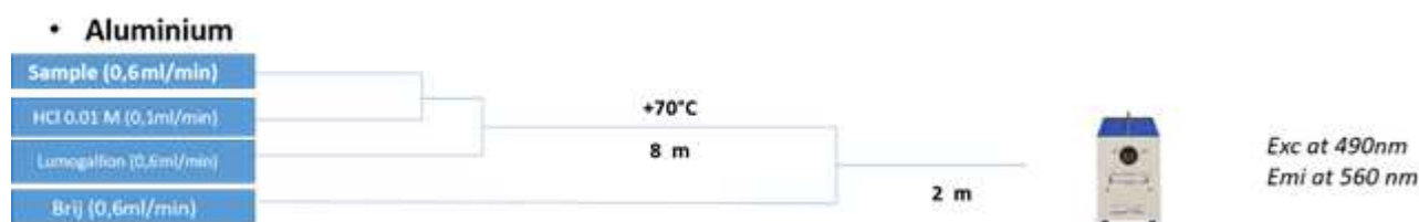
Figure 24 - Analytical set-up for the soluble Al method
