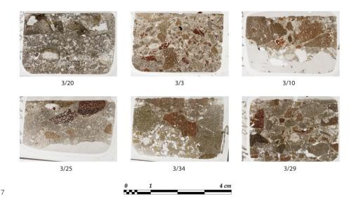
Fig. 7: Selinous. Thin sections of the concretes
