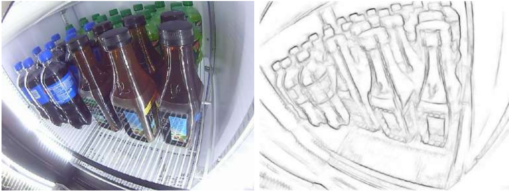
Figure A.3: Example of the edge detection results: the original shelf image on the left and the edge image on the right.
