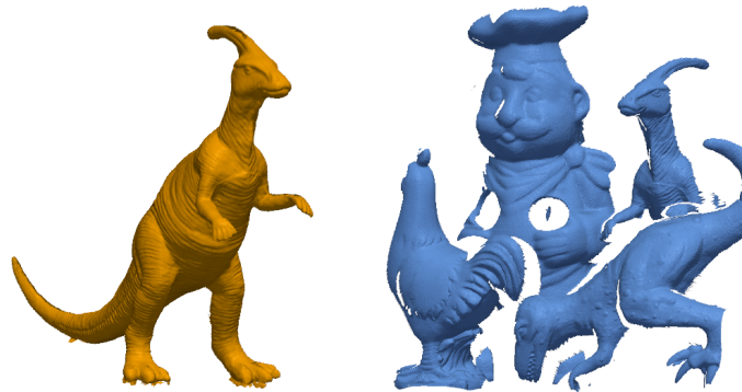
Figure 2.4: A typical 3D object recognition scenario. Clutter of the scene and occlusion due to the geometry of the ranging sensor seriously hinder the ability of both global and feature-based techniques to spot the model.
