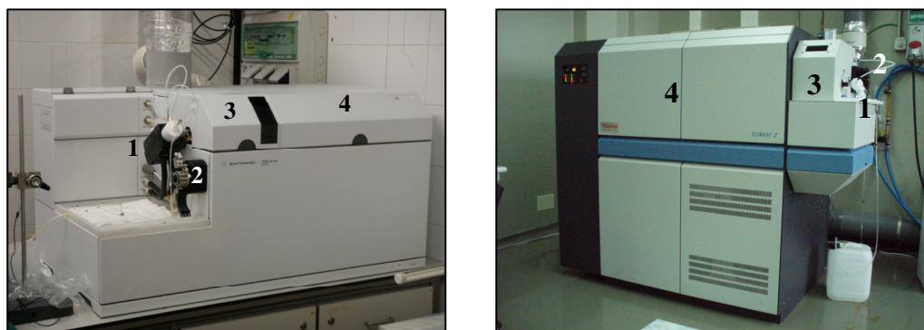
Figure IV-2 Pictures of the ICP-MS Agilent 7500cx (left) and Thermo Element2 (right): 1) spray chamber assembly; 2) peristaltic pump; 3) ionization compartment; 4) mass analyzer compartment.
