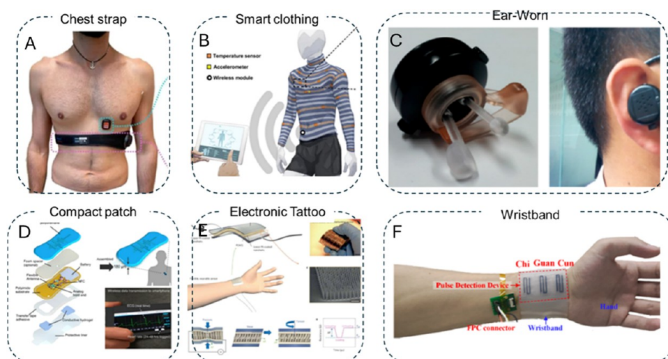
Figure 34. Soft wearable heart rate monitoring devices. (A) Chest strap ECG sensor. Reproduced from Romano et al. 797 Available under a CC BY 4.0 license. © 2022 MDPI. (B) Smart clothing with PPG sensors. Reproduced from Wicaksono et al. 654 Available under a CC BY 4.0 license. © 2020 Springer Nature. (C) Ear-Worn Piezoelectric Sensor. Reproduced from Park et al. 804 Available under a CC BY 4.0 license. © 2015 MDPI. (D) Compact patch integrating ECG sensor, signal processing, and transmission module. Reproduced from Lee et al. 789 Available under a CC BY 4.0 license. © 2018 Springer Nature. (E) Epidermal electronic heart rate device based on triboelectric Sensors. Reproduced with permission from Pang et al. 750 © 2012 Springer Nature. (F) Wristband pulse sensor-based piezoresistive technology. Reproduced from Wang et al. 801 Available under a CC BY 4.0 license. © 2022 MDPI.
