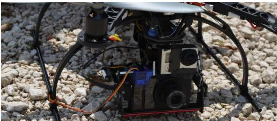
Fig. 38: la fotocamera compatta Canon Powershot S100 e la *action camera* GoPro Hero3 Black Edition.
