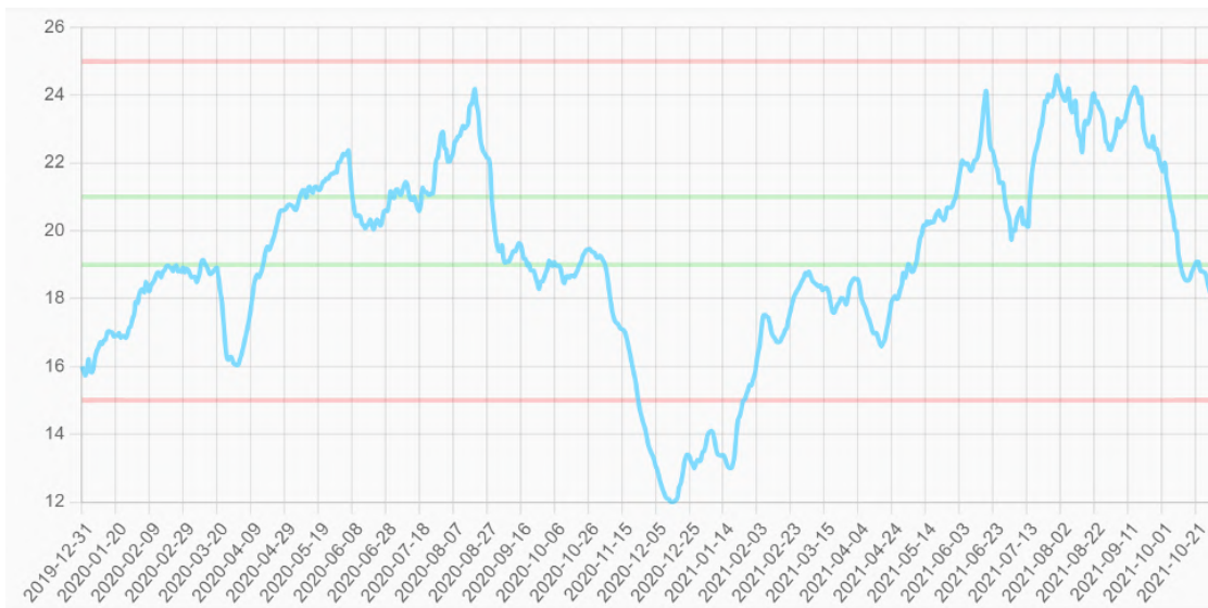
Figure 4.14: Temperature data obtained from the sensor inside Hasan cloak display case container
