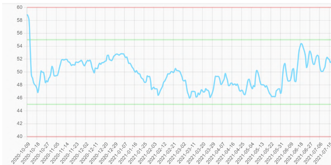
Figure 4.49: Relative humidity data obtained from the sensor inside Mur Breton container
