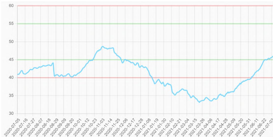
Figure 4.25: Relative humidity data obtained from the sensor inside Collection of historical photographs container
