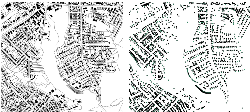
Figure 8 Land parcel and structure locations on the GIS map in the Harbor case study area. Property outline and building position (left) are used to derive the centroid point of each parcel of land (green dot) and each structure (black dot) to collect elevation information for the analysis.
