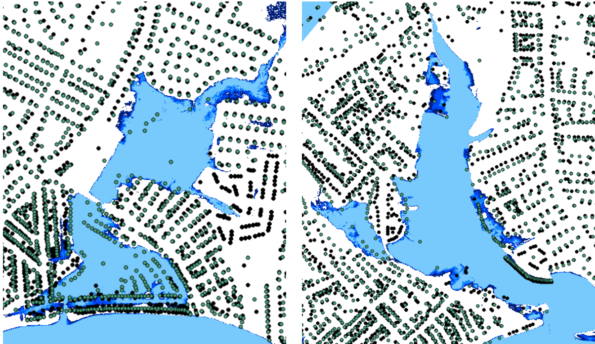
Figure 16 GIS maps of sea level rise at MPST in 2025, 2050, 2075, and 2100 in the Bayview (left) and Harbor (right) case study areas. Green dots represent the center point of each parcel of land and black dots represent structures.
