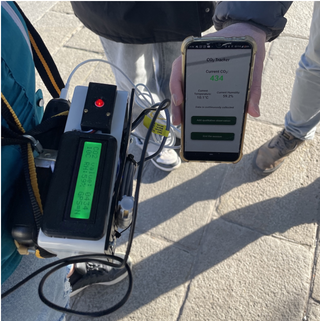
Figure 6: The mobile station and the smartphone connected to the web application display the same data on their visual interfaces.
