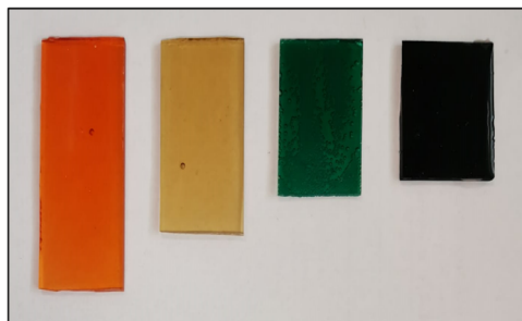
Figure 5. Examples of dyed samples of polyesters obtained by the reaction of glycerol with CLM. Conditions of prepolymerization and curing were those of Figure 4.
