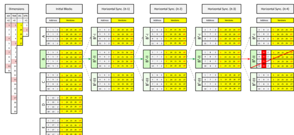
Fig. 23 Map of transmitters and receivers with entries considered for each iteration. Each set of nodes depends on the cell selected for the synchronization in the previous step
