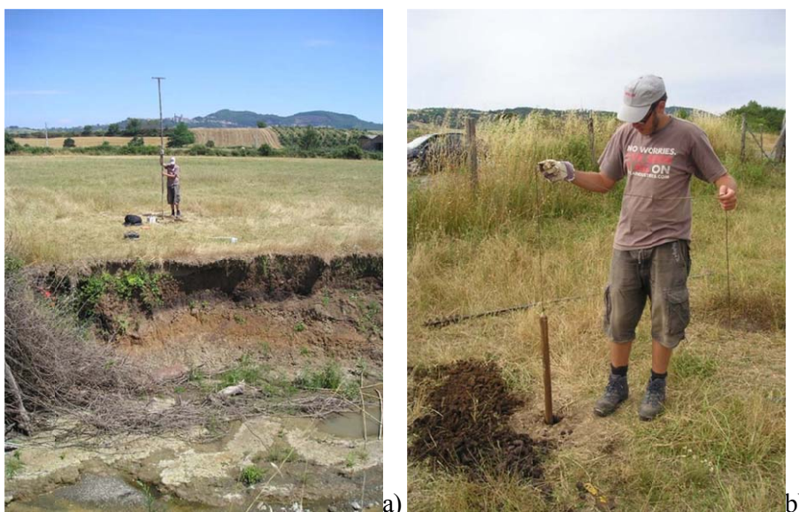
Figure 65. Photographs showing the full length of the auger after drilling of P3 in the pasture field south of the emanation area (a), and use of a bailer to clean muddy water from a hole prior to pumping(b).
