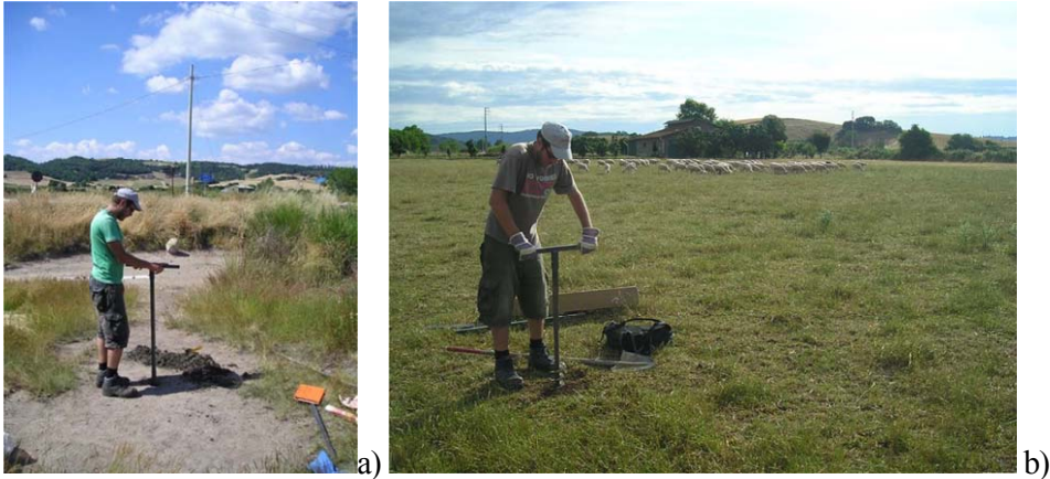
Figure 62. Photographs showing the difference in surface appearance, within the area of highest gas emission (a) and about 500 m to the SW in a pasture field with no leakage (b). For locations of piezometers P1 (a) and P5, see Figure 64a.
