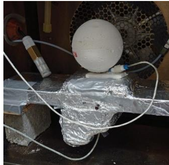
Figure 2.1: Experimental setup inside the GC HP 5890 series II oven. The spherical mortar specimen is placed on a needle-shaped thermocouple, while another is attached on the side for the surface measurements. The white sensor on the left is used to measure the temperature (T) and relative humidity (RH) throughout the experiment.
