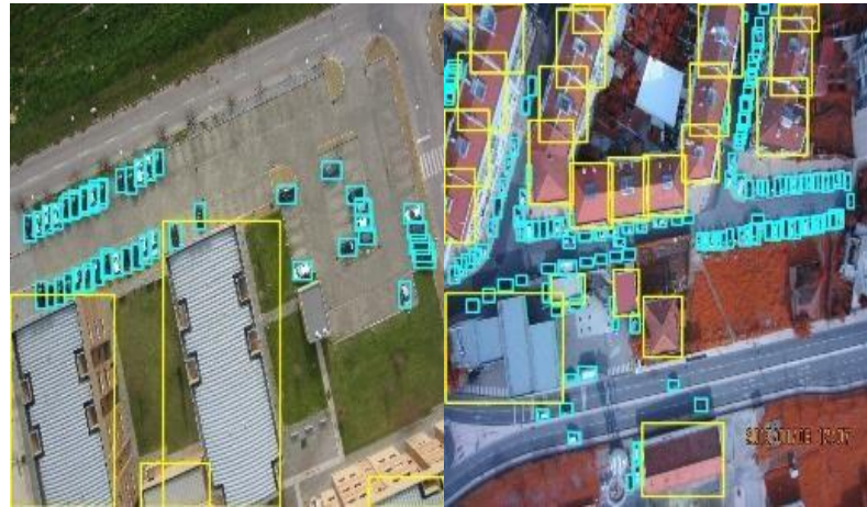
Figure 1 – YOLOv5l algorithm detection results for two images from the PMA dataset, captured in a UEO of Portuguese Army
