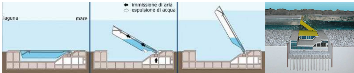
Figure 2.9 Functioning of the floating gates (first 3 figures from the left) and cross-section of the gates and the housing buried in the inlet bottom (on the right)
