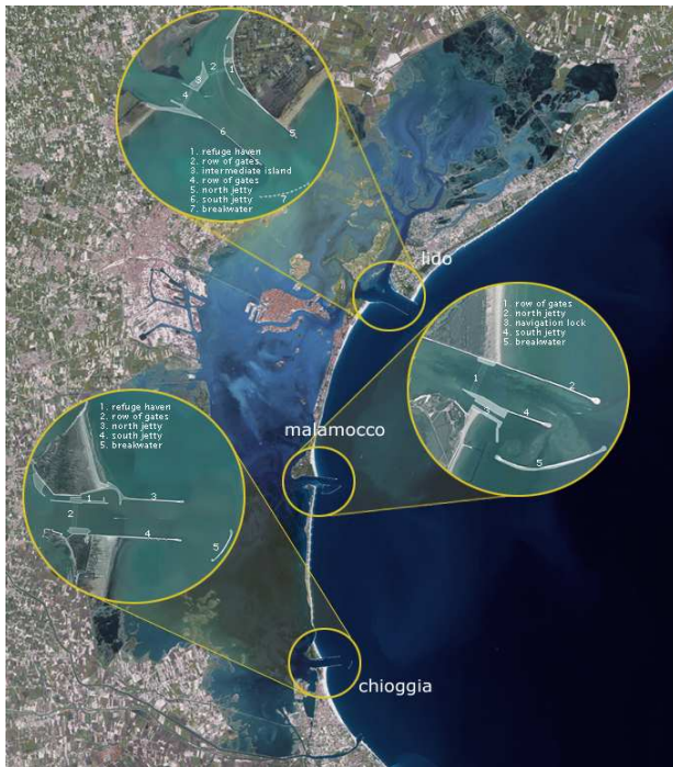
Figure 2.8 Project design of the mobile barrier system to protect Venice from tidal floods (MOSE)
