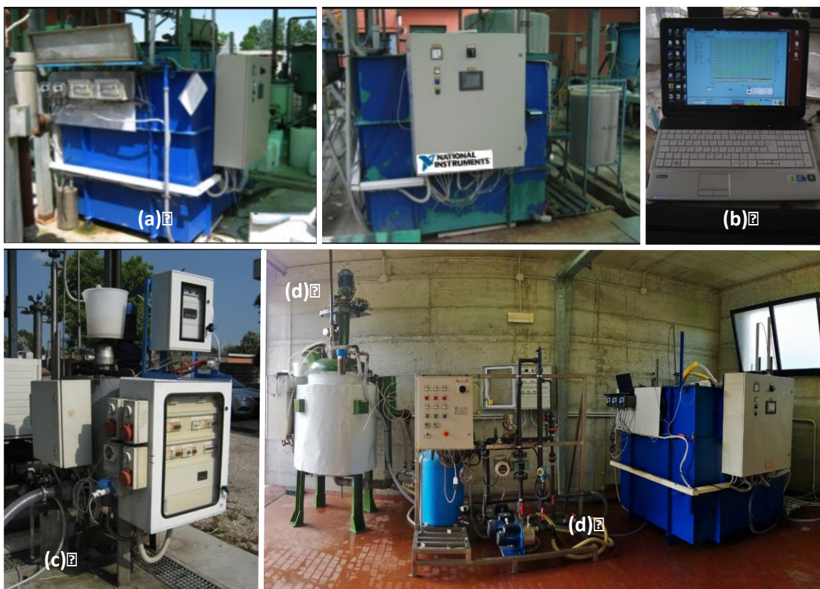
Figure 3.2. a) Pilot Sequencing Batch Reactor with 2.8 m 3 of working volume for the treatment of anaerobic effluents; b) Graphic interface to monitor and control the pilot SBR; c) fermentation
