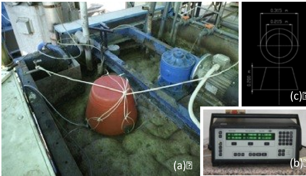
Figure 3.5. View of the SBR and floating container for the on line gas measurement, (b) instrument for the on line measurement of gas emissions and (c) cross section and side view of the floating container.
