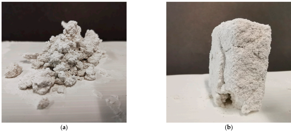
Figure 6. (a) MSCL025 sample after 6° saline cycle; (b) MSD025 sample after 8° saline cycle.
