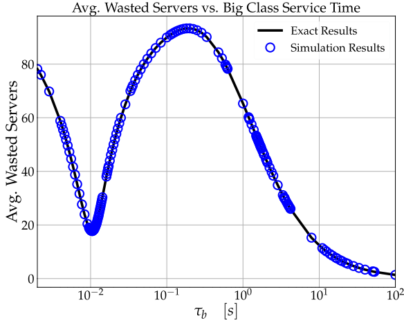
Fig. 4. Average number of servers wasted because of HOL blocking in a saturated MJQM-FIFO with small and big jobs versus average service time of big jobs. N = 200 , small jobs request 1 server, big jobs request 100 servers, \tau_s = 1 , p_s = 0.5 . Comparison of simulation predictions against the exact analytical results of [3], [4]. The y -axis scale is linear.
