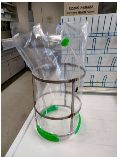
Figure 30: Example of benthic chamber structure
