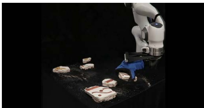
Fig. 1 – The robotic arm moves the wall painting fragments of the Casa dei Pittori a lavoro (Pompeii; photo credit: RePAIR Project).
