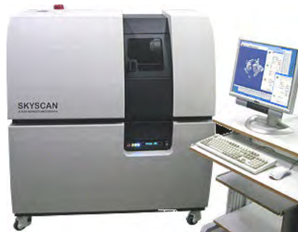
Figure.11. X-ray \mu -CT set-up SkyScan 2011 used at Geomodel Research Centrum of Saint-Petersburg State University.
