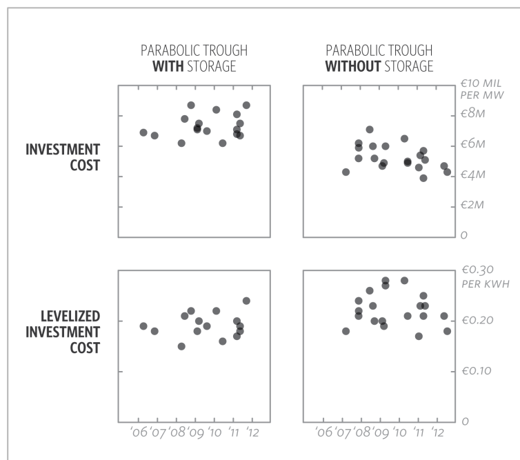
Figure 2: Investment and levelized costs for parabolic trough plants between 2006 and 2012 – Source: Author
