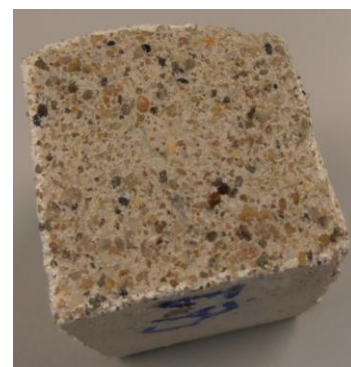
Figure 3.3 14 wettability behaviour of the inner core in comparison to the outer side layers in a PM7301 specimen
