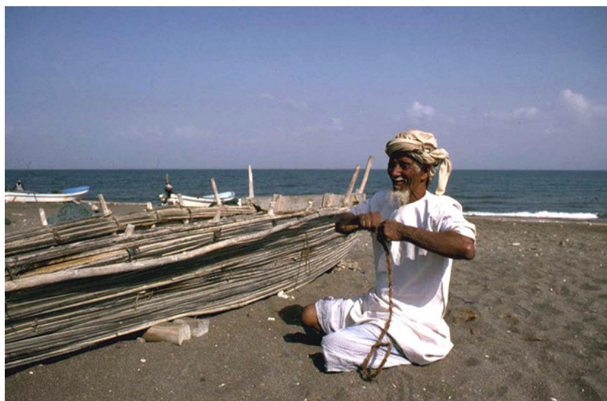
Fig. 15 An Omani fisher repairing a traditional shasha boat made from reeds at Barca, along the Batinah coast of the Sultanate of Oman (photograph by P. Biagi 1989)
