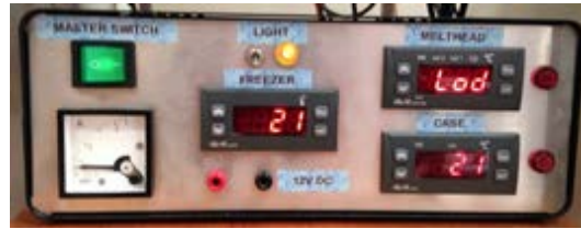
Figure 4.3: Frontal view of the controller. The freezer , melthead and case temperature sensor displays. On the left: the heating cartridges current display.
