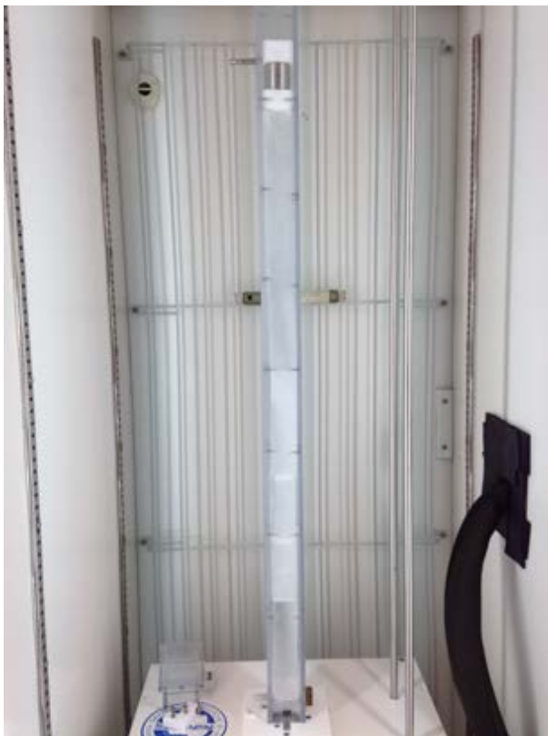
Figure 4.9: The holder in the freezer filled with a core section placed on the melting head.
