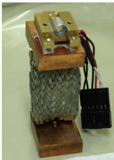
Figure 3.1: The SP2 Nd-YAG crystal, its support and power supply connections.
