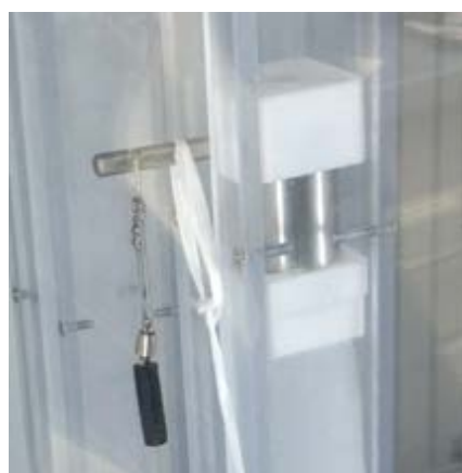
Figure 4.5: Connection between the draw-wire sensor cable and the weight in the holder.
