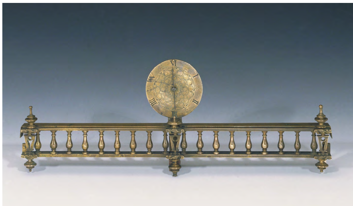
Fig. 9. Paper-ribbon hygrometer improving on Folli's design, most probably by Gio. Filippo Treffler (1666). Florence, Museo Galileo, Inv. 2435.
