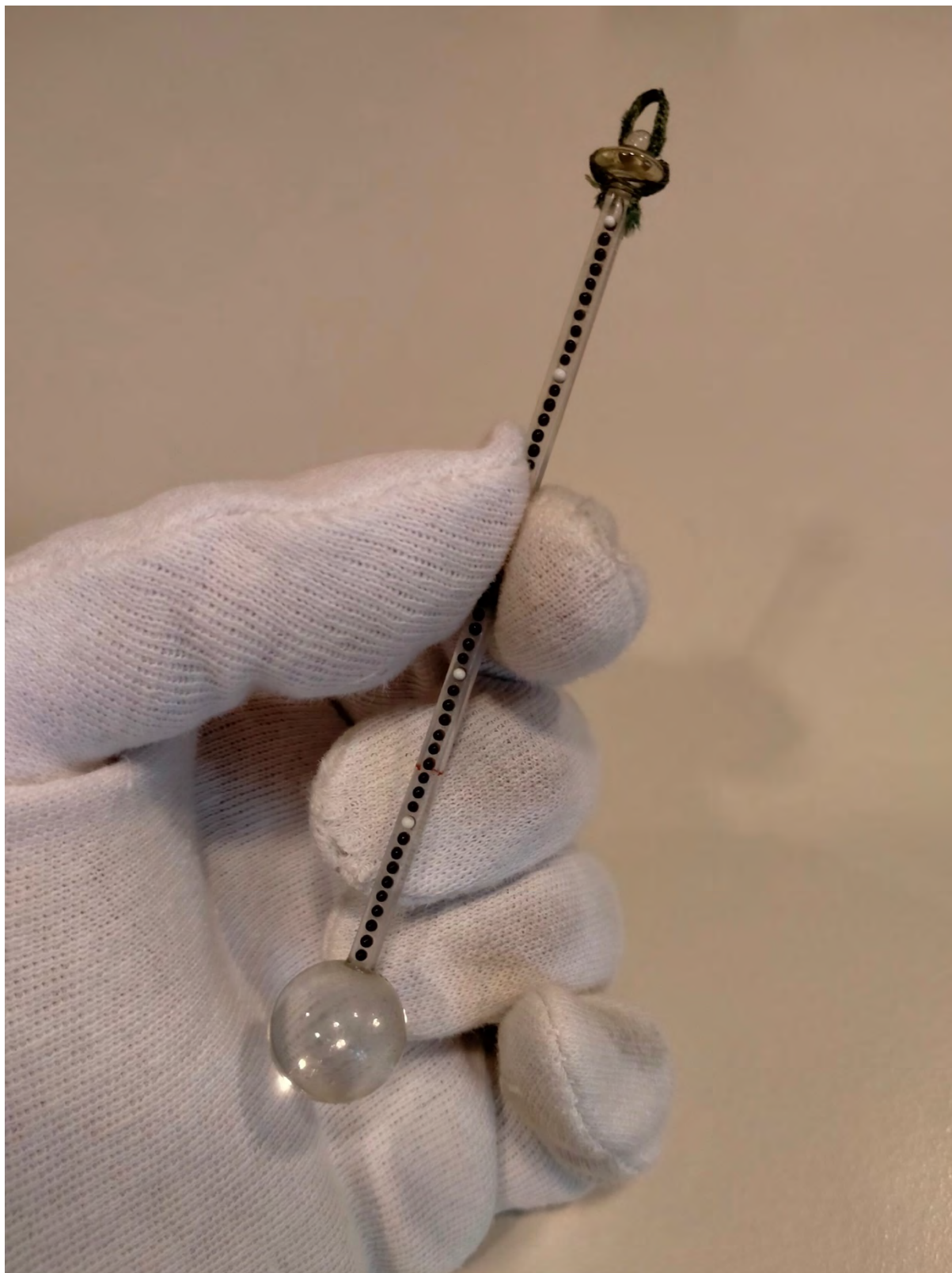
Fig. 2. A 50-degree thermometer invented by Ferdinando II and made by the Gonfia. Museo Galileo, inv. 31-64.
