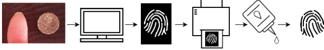
FIGURE 2. Schema of the fingerprint forgery process adapted from [12]: (1) a finger-photo, (2a) template preparation – extracting papillary lines, (2b) inverting colors on the template, (3) printing the mold on the printer (4a) application of a cast material on the mold and (4b) resulted counterfeit.
