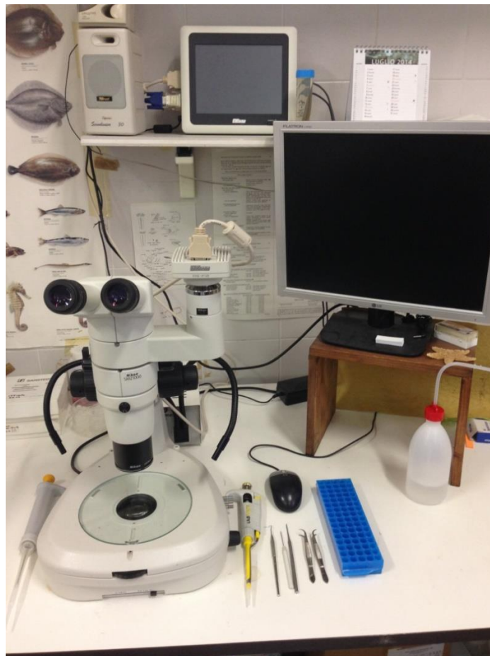
Figure 33 – Stereo-microscope (Nikon SMZ1270) and high-performance camera (Nikon DS-Fi2) coupled with a digital controller (Nikon DS-L3).
