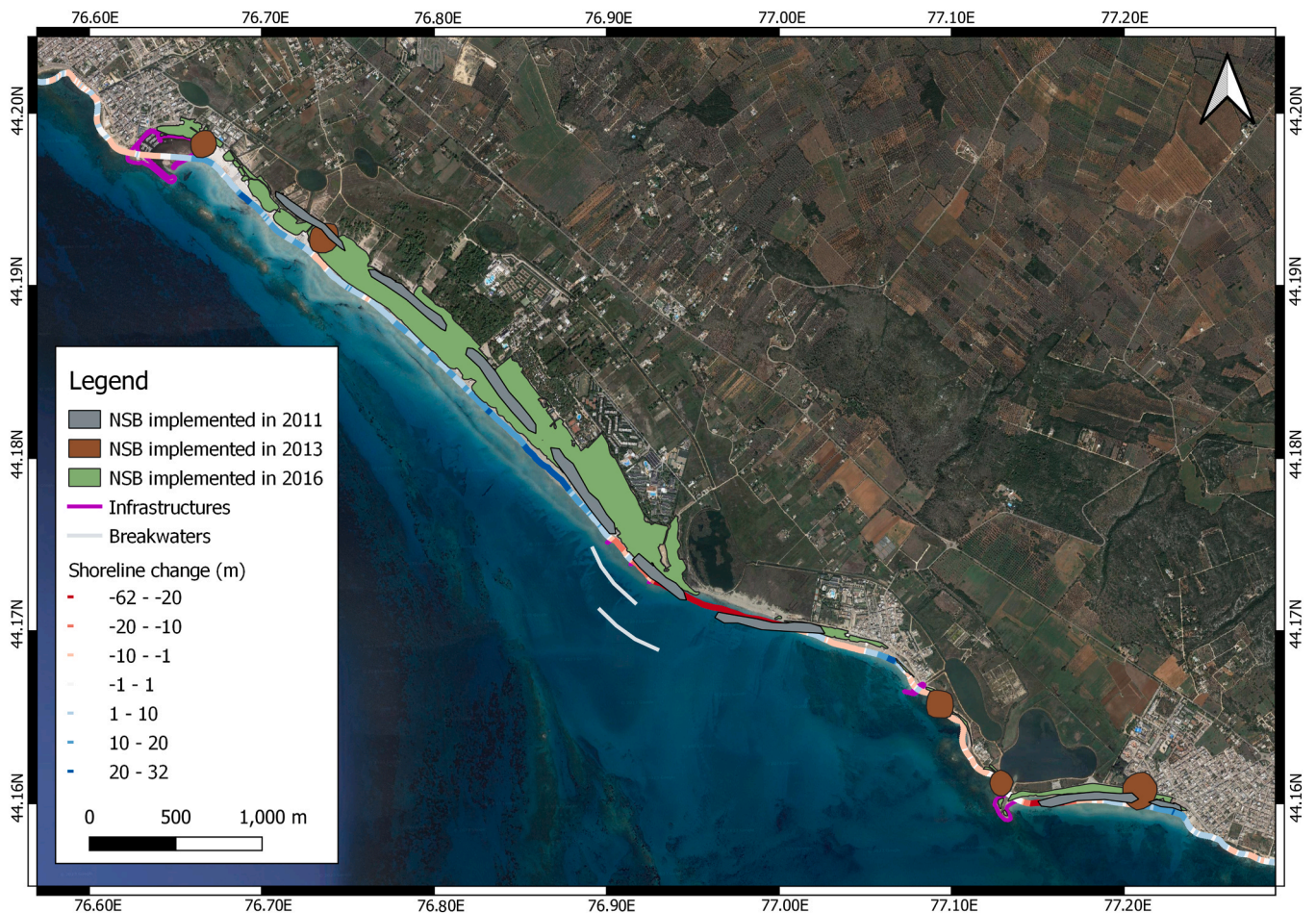
Fig. 8. Spatial representation of the NSM indicator against the management measures (i.e., NBS, breakwaters and infrastructures) implemented during the investigated timeframe (2009–2018).
