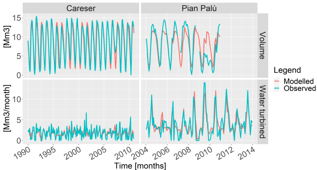
Figure 15 -. Careser and Pian Palù dam reservoir volume stored and water turbined for their baseline periods (x scales are different)
