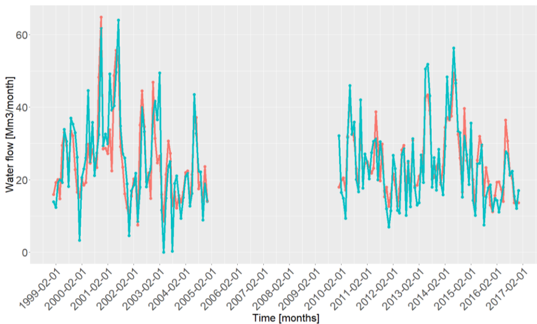
Figure 6 – S.Giustina time-series of water diverted to the turbines. Measured (blue line) and modelled (red line) water outflowing from the S.Giustina dam reservoir from 1999 to 2017. R^2 = 0.79 , RMSE= 4.7
