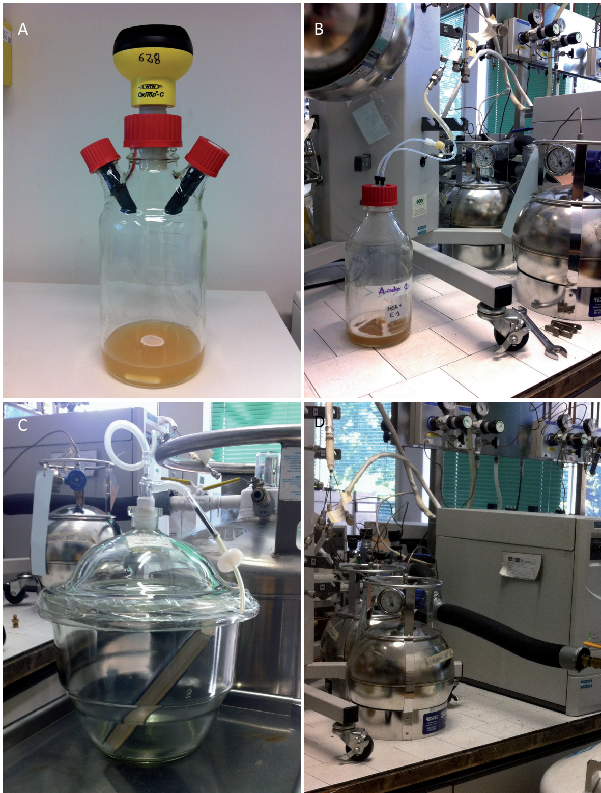
Figure 3.6 Sampling techniques: A: Sample bottle for BOD analysis; B: Sampling bottle for MVOC analysis from pure fungal colony; C: Sampling chamber for MVOC analysis from contaminated book; D: Air sampling by canister between shelves.
