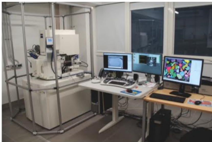
Figure 10: the SEM at Milan-Bicocca University (original figure by Brochure-TECLA.pdf of Milan-Bicocca University).
